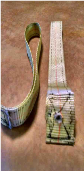
Double the strap then sew the two ends together at one end. You will secure this end to the bolt under the hood.
